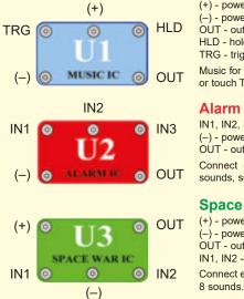
(+) - power from batteries (-) - power return to batteries OUT - output connection HLD - hold control input TRG - trigger control input Music for ~20 sec on power-up, then hold HLD to (+) power or touch TRG to (+) power to resume music.
