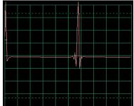
The waveform above is weak and erratic, so replace the  $0.02\mu$ F capacitor (snap part C1) with the  $0.1\mu$ F capacitor. A sample of the new waveform is at left, with the same settings. It is lower in frequency but higher in amplitude.
