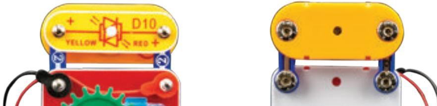
Modify the preceding circuit to include the red/yellow LED (D10) and melody IC (U32), mounted on the car using two 2-snap wires. A tune plays and the LED lights yellow when the car is going forward, or the LED lights red when the car goes backward-turning.
